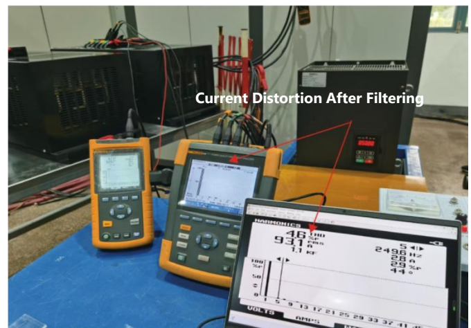
After filtering of TSHF harmonic filter THDi=4.6%
