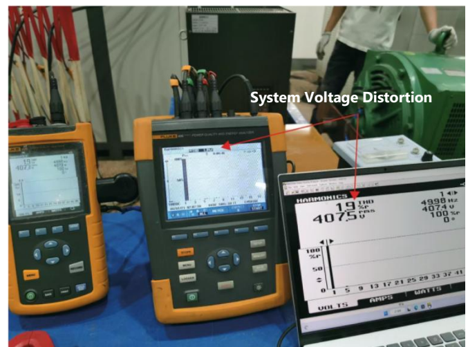
System Voltage Distortion in Frequency Converter Testing THDi=1.9%
